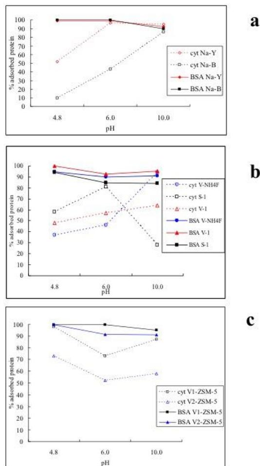
**Figure 4.** Influence of pH on BSA and cyt c adsorbed on different zeolite supports: (a) Na-Y and Na-Beta, (b) V-NH<sub>4</sub>F, S-1 and V-1, (c) V1-ZSM-5 and V2-ZSM-5.
