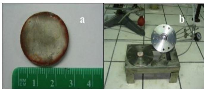
Figure 1. Images of Na-Beta zeolite composite membrane and (a), and the experimental permeation cell used in this work (b).
